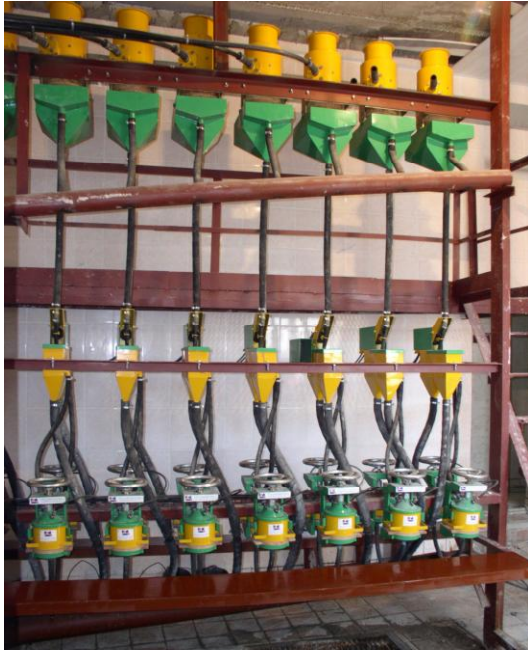
The photo of the sample delivery system “Kontur” and the control box with the “Ge Fanuc” controllers. This system is developed for Kaztsink Corporation (Kazakhstan).
